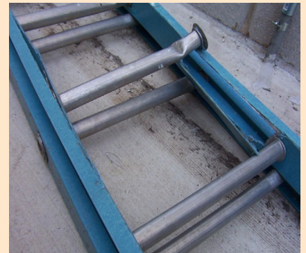
Remove damaged ladders from use.
