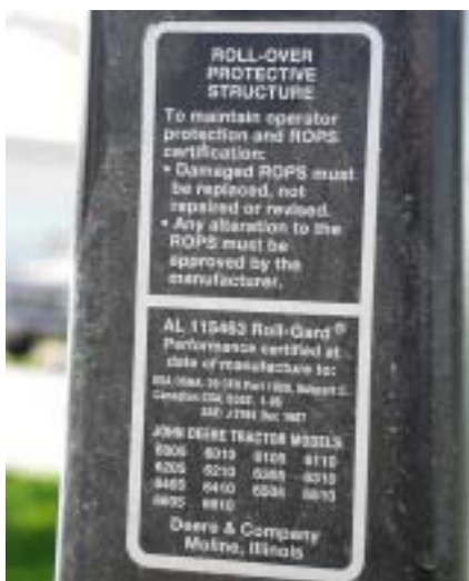
Figure 4. This certification tag indicates the ROPS meet nationally approved standards for operator protection during a rollover.
