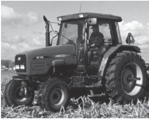
Figure 2. A ROPS with enclosed cab gives the operator the most protection from common hazards of tractor operation.
