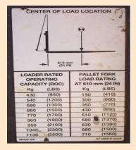
Know load center and capacity information to avoid machine tipover or failure.
