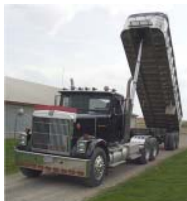
Figure 1: Raised beds of large farm dump trucks and trailers present several possible hazards.
